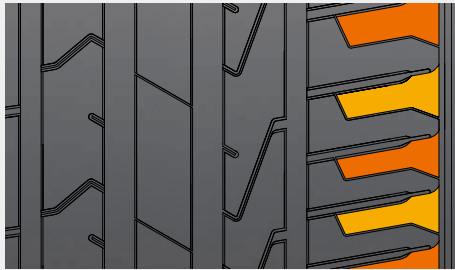
Noise reduction through an optimised pitch design.
